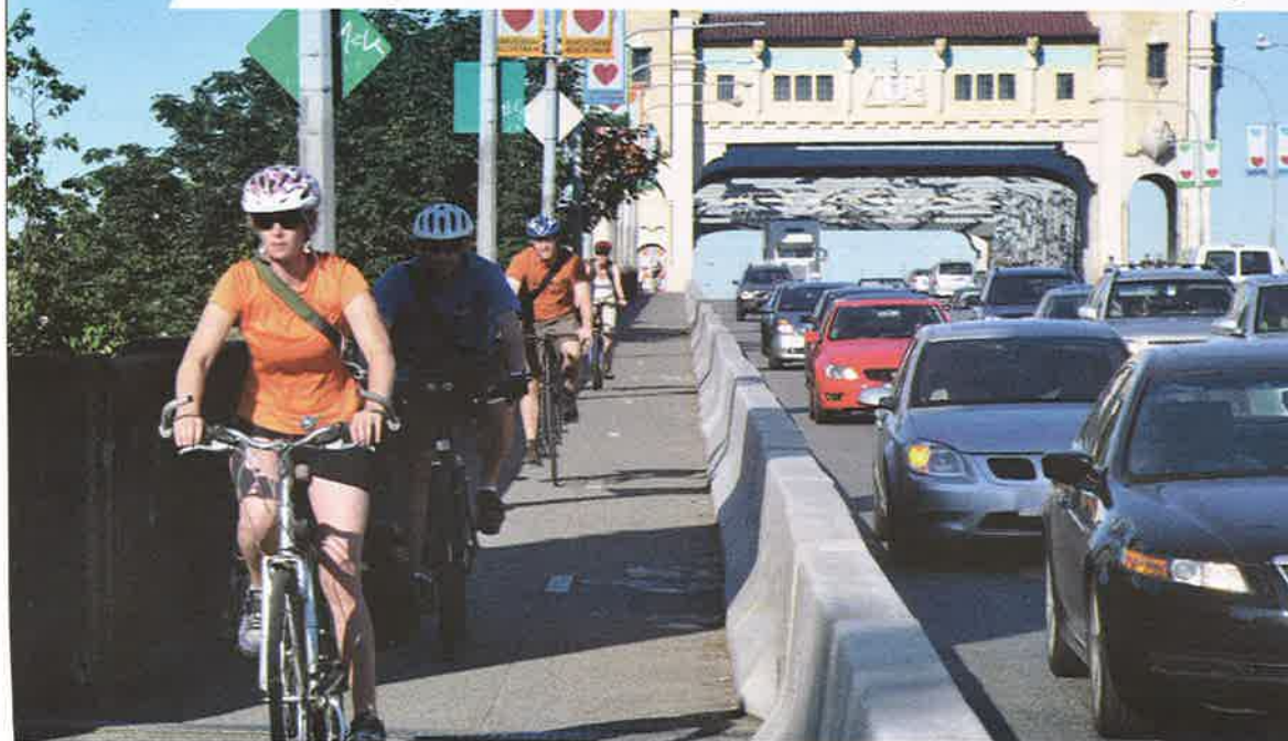
Riding across the Burrard Bridge in the cycling lane, protected from automobile traffic. During peak periods, between 500 to 800 cyclists cross the bridge every hour. Photo courtesy of City of Vancouver
