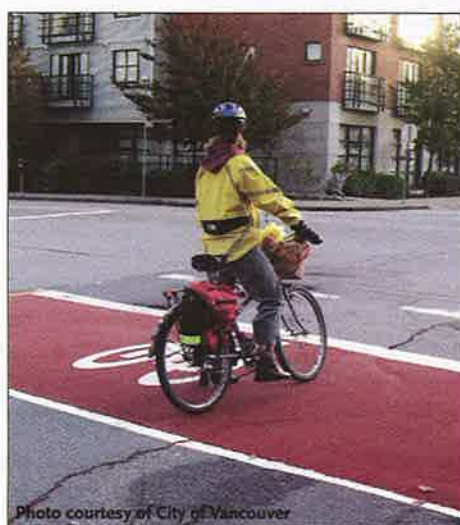
Bicycle boxes allow cyclists to go ahead of motor vehicles, providing better visibility.
